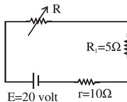
**STATEMENT – 2 :** Since  $R_1 < r$  in the given circuit. So, power transfer in external resistance will be maximum when  $R = 0$ .
