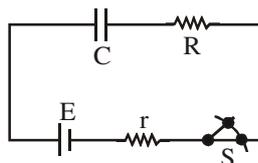
**STATEMENT – 2 :** Initially capacitor was uncharged, so resistance offered by capacitor at  $t = 0$  is zero.
